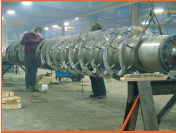
Reinforced support stanchions installed to reliably hold ribbon flighting.
