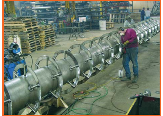
Conveyor screw is ground and polished to meet customer requirements.
