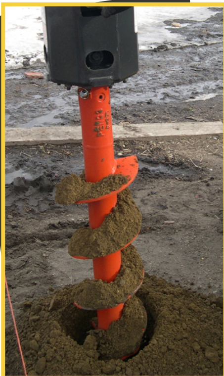
Pictured Left TriMax® Auger with 37 Gage and 5T30 Fas-N-Lok® Teeth drilling in frozen soil.
