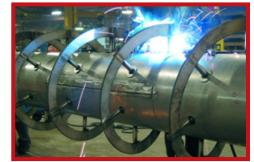
Reinforced support stanchions installed to reliably hold ribbon flighting.
