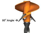
AGGRESSOR® auger teeth are for use in dirt, abrasive soil or fracturable rock, depending on the type of tooth you are using. All types of the 40/50 tooth can be used at either a  $40^{\circ}$  or  $50^{\circ}$ angle providing different attack angles based on your drilling condition.
