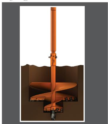
Pengo's Aggressor® tree auger is a robust version of our Landscape Aggressor® Tree Auger and made specifically high-duty cycle applications. Offering the same two-stage design that produces a tailored fit for the root ball, the Aggressor® also offers the options of a 2" hex connection and the ability to change the pilot and teeth to accommodate light rock and permafrost soil conditions.
