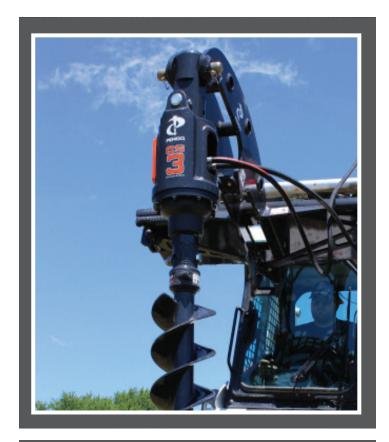
Pengo's latest addition to the Revolution Series Drilling drives are the CS Models. These models compact and light weight and are designed to work with our General Purpose 2" Hex Aggressor®, TriMax® and Severe Rock Ripper® augers. Combining this drive with the CS-3 Mount and your Pengo auger gives you a complete auger package.
