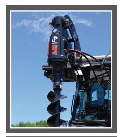
Pengo's latest addition to the Revolution Series Drilling drives are the CS Models. These models compact and light weight and are designed to work with our General Purpose 2" Hex Aggressor®, TriMax® and Severe Rock Ripper® augers. Combining this drive with the CS-3 Mount and your Pengo auger gives you a complete auger package.
