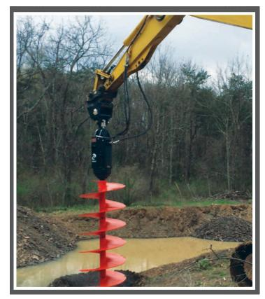
The High Speed DV-30 Drive is compatible with Pengo's Excavator Auger system. The drive will drill holes up to 20' deep and 6' in diameter in rock, dirt and frozen ground.
