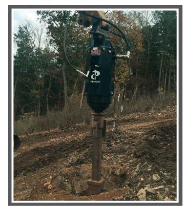
The DV-40 is the largest drilling drive in the Revolution Series. This drive with turn Pengo Excavator augers 25' deep and as wide as 7' in diameter. Like the DV-30 it is able to drill in most rock, dirt and frozen ground drilling conditions.
