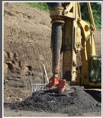
The PENGO foundation dirt augers withstand the rigors of your job. Both double cut, single carry and double cut, double carry augers feature the TriFlow® pilot bit and taper-fit dirt teeth.
