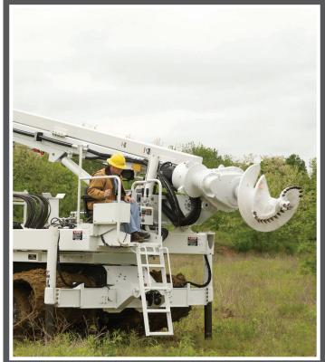
Pengo® True Cut PDR augers are made with thick, heat-treated cast alloy heads and Pengo's own STRATA® SR-100 conical teeth. The cast heat treated head provides superior wear and performance compared to normal fabricated augers. In addition the cast head is field repairable with standard welding techniques, utilizing low hydrogen welding rods and no pre- or post-heating requirement.
